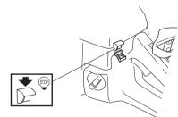
The engine is stopped by pushing the stop switch to the stop position.
